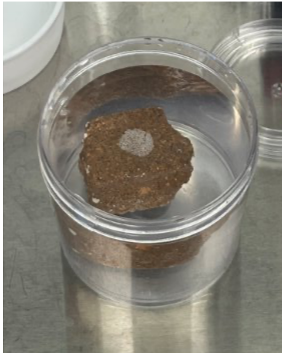
Picture 1. Paver with Sealant testing for efficacy
